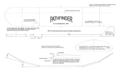
PATHFINDER 16" span 5 panel wing with a 3" chord. Simple outlines , easy construction. The straight airfoil high point line makes for easier shaping. **Many Wins** including the 2009 Nationals. Great launch height. Includes RR fuselage with built in viscous timer.
