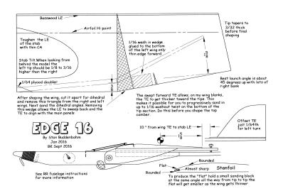
EDGE 16's wing shape and construction method makes for easy but advanced shaping of the airfoil. The wing is shaped while the LE is straight and the TE is swept forward. Then a section is cut out to give the final LE swept back plan form. See the latest Stanfoil page for shaping details. Several contest wins in 2016. Kit includes the RR fuselage with built in viscous timer.
