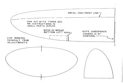
OBARSKI is old time SAM legal. 18.75" span, 3.5" chord. The kit fuselage is a balsa version of the RR fuselage with my built in viscous timer and matches the original fuselage to maintain its legal status. This kit won both Old Time Cat and Old Time Hand Launch Glider at the 2014 Nationals.
